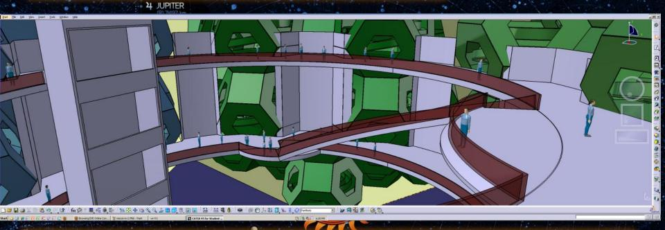
Brady and I are still deciding how to build this, but this preliminary visualization gives a sense of how the proportions and distances work, which is mainly what I need. Communications between the levels will mostly be by six helixes going up the atrium, enclosed in steel netting for safety, with low-incline ramps and then a few seats like ski-lifts along the side.
